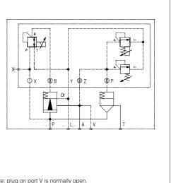
Note: plug on port V is normally open. V port can be used for optional connection to a solenoid valve for venting.
