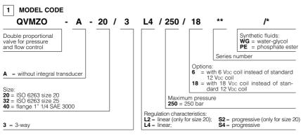
QVMZO are double proportional valves, which provide the indipendent flow and pressure control in systems with fixed displacement pump, according to the electronic reference signal.
